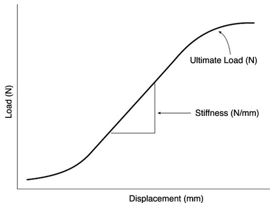
**Fig. 3** Schematic load-deformation curve defining stiffness (N/mm)
