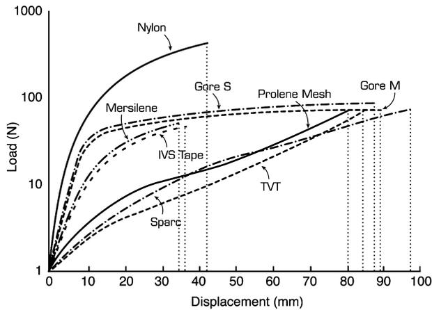
**Fig. 4** Typical load-deformation curves for the eight tested permanent materials (log scale). The vertical dotted lines indicate the displacement at which failure occurred
